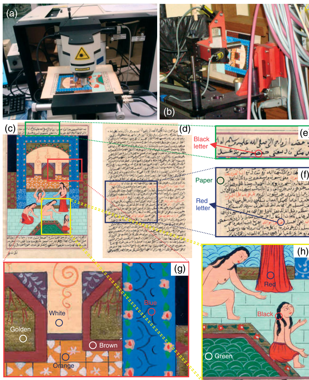
Figure 1. Photographs: (a) micro-Raman system setup; (b) XRD/XRF portable system setup; (c–h) illuminated manuscript showing the measurement zones (and magnifications, e–h).
