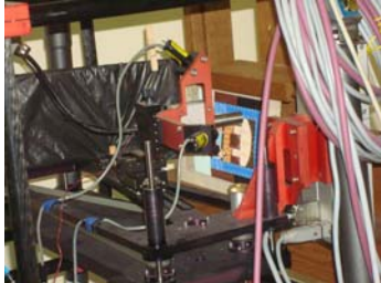
Experimental set-up of the XRD/XRF portable system employed by manuscripts analyses
